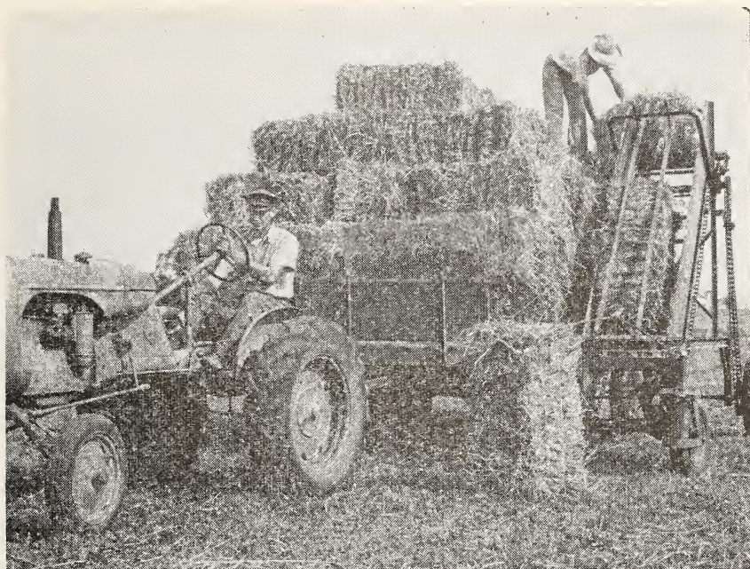
FIGURE 19.—This field bale loader picks the bales up where they were dropped by the baler. It elevates them to the top of the load and eliminates much of the strenuous labor associated with the loading of bales from the ground.
